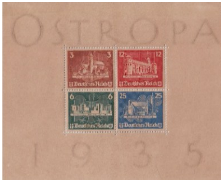
Ostropa sheet with paper breaking down and discolored by acidic stamp gum.
