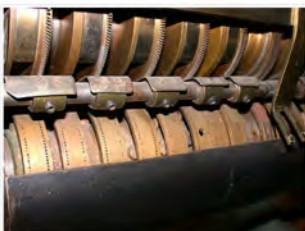
Close-up of the National Postal Museum’s machine, showing matching sets of pins and holes
